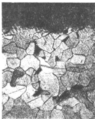
Fig. 4. Twins in ferrite grains at the edge of the cavern. \times 400 .
